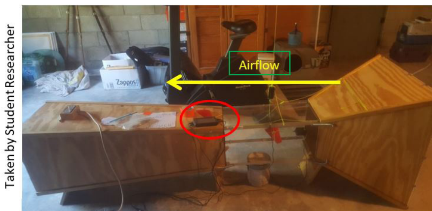
Figure 6: Wind tunnel design. The right-hand side is where the wind tunnel collects air and the left-hand wooden compartment houses the fan. The clear section in the middle is where the models were observed and tested.
