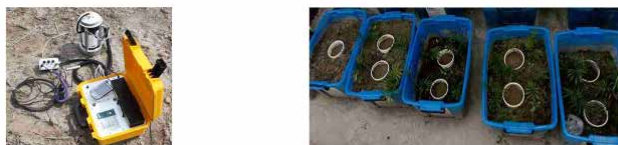
Figure 10. Soil respiration test instrument and test process: a) left is the soil respiration test instrument, b) right is breathing ring
